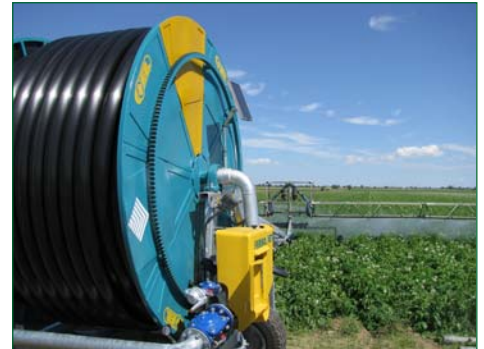
Hose reel machine using spray boom
