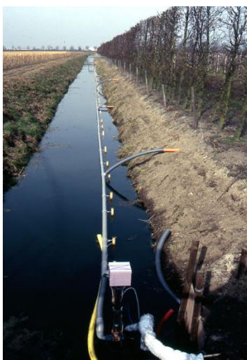
Figure 11. Field research on the discharge of chemicals through subsurface drains under apple trees in relation to the application
