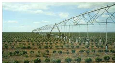
A centre pivot irrigating young coffee plants in Brazil (Almost half of Brazil's 3.44 mha of irrigated land is under pressurized irrigation, and over 40% of that is under centre pivot)
