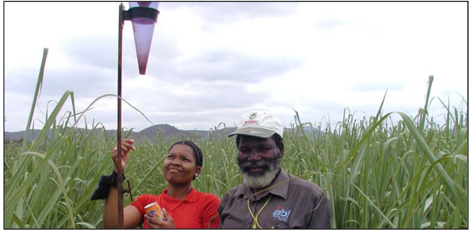
Mr. Mthembu and his daughter measuring water applied through sprinkler irrigation in their sugarcane field in Pongola, South Africa
