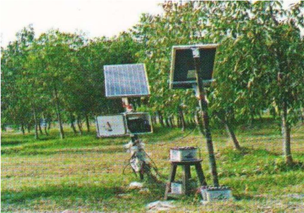
**Figure 6.** Measurement of transpiration rate with sap-flow meter
