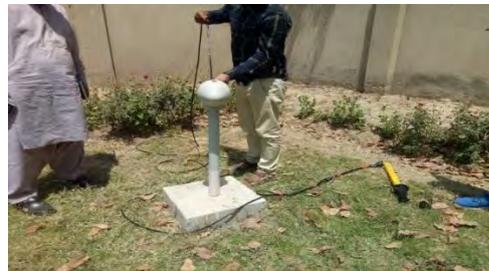
**Figure-6:** CTD sensor installed at Jalwala head (ESC Tail)
