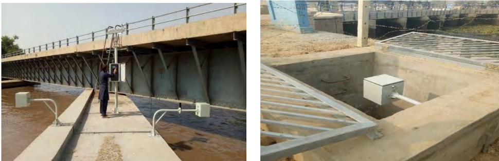
**Figure 4:** RTFM Sensors installed at Eastern Sadiqia & Fordwah Head at Suleimanki Barrage and at Jalwala Head
