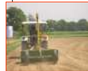
Laser land levelling to reduce GW draft by 19 cm Rice-Wheat areas in Punjab (Applicable to Yamuna Alluvial Plains)
