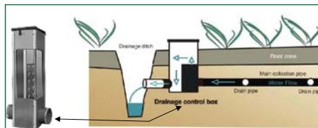
**Figure 2.** A control structure used with buried drain lines.
