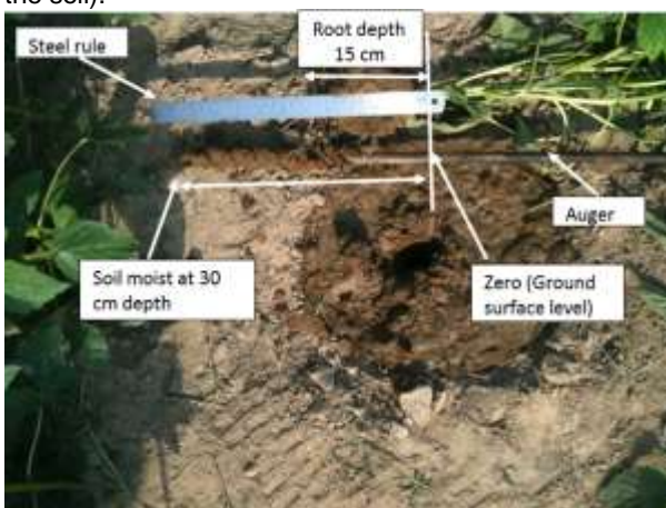
(e) Soil water infiltrated 30 cms, root boll of sesame crop was 15 cms
