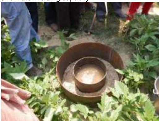
(a) Identifying the soil type and thus the infiltration rate and water holding capacity
