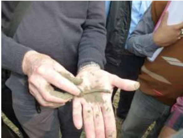
(a) Identifying the soil type and thus the infiltration rate and water holding capacity
