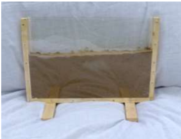
(a) A perspex sided display cabinet for demonstrating infiltration rate in soil. The cabinet is filled with sand and water poured onto the top of the sand. The rate at which the water infiltrates into the sand can then be viewed.
