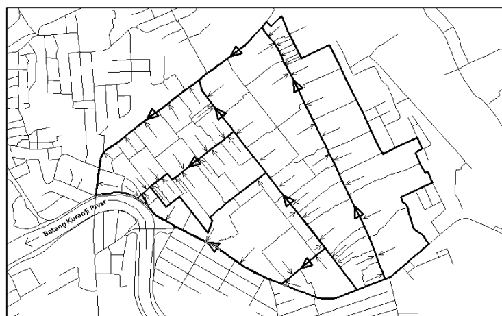
Figure 5. Drainage canal layout
