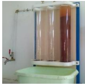
Figure 1. Infiltration demonstration apparatus
