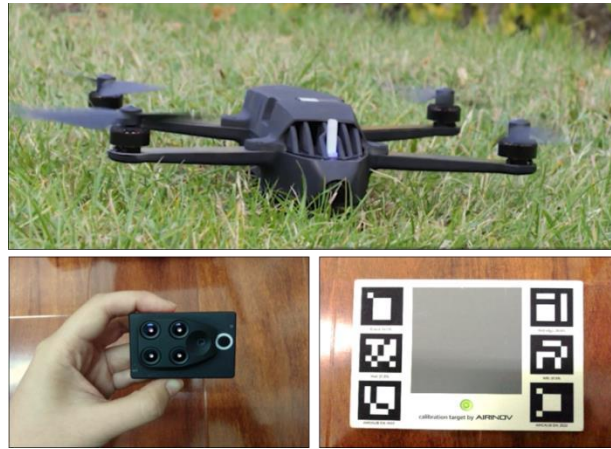
Figure 2. UAV-camera system: Parrot Bluegrass UAV, Parrot Sequoia camera and reflectance panel.
