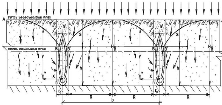
**Figure 4.** Design model to identify the distance between the drains
