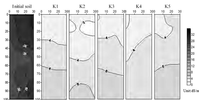
**Figure 3.** The spatial distribution of EC<sub>e</sub> in the vertical transects perpendicular to the drip lines before transplanting rose and in November 2014
