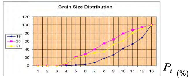
**Figure 6.** Grain-size curve – (21) soil depth – 0,30 m. (20) – soil depth – 0,50 m. (19) – soil depth – 1,0 m.
