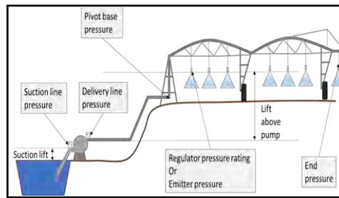
**Figure 1.** Diagram showing the locations where system pressure is measured to determine system efficiency and diagnose energy losses.
