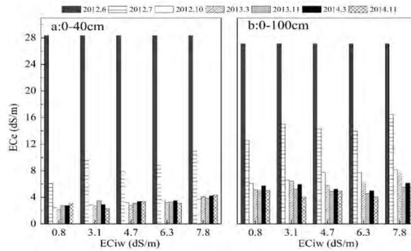
**Figure 4.** The average  $EC_e$  values of 0-40 cm (a) and 0-100 cm (b) soil profile during the experimental period
