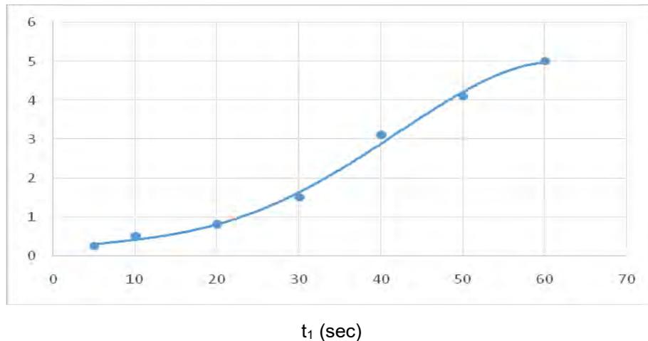
**Figure 8.** Graph of dependence  $Q_1 = f(t_1)$  for the first drainage pipe.
