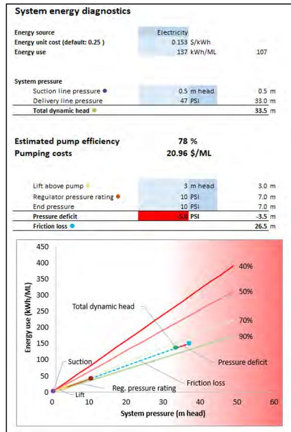
Figure 4. System energy diagnostics output used to assess pumping efficiency for Case study 1
