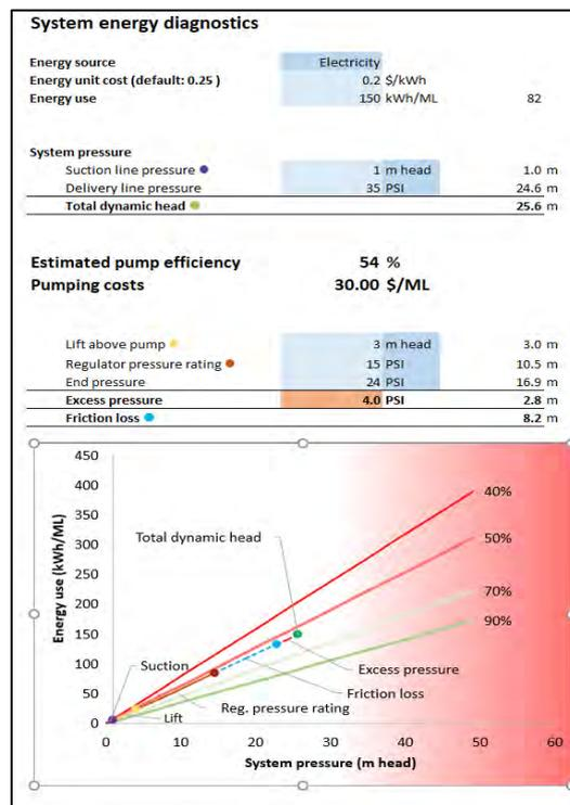
Figure 6. System energy diagnostics output used to assess pumping efficiency for Case study 2
