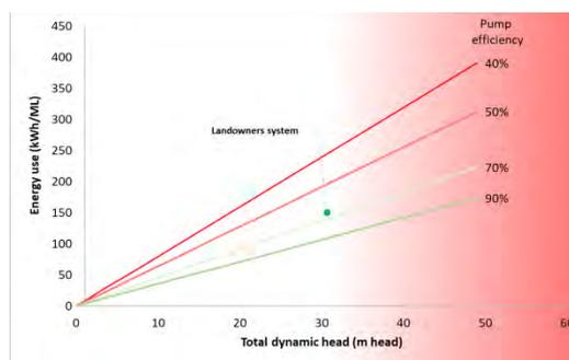
**Figure 2.** Graphical output from the Energy Calculator showing the Total dynamic head and Energy use of the landowners irrigation system plotted against pump efficiency isolines.
