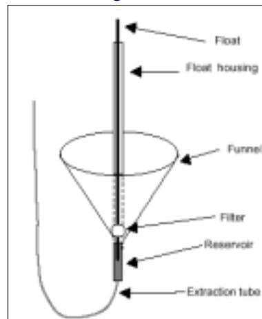
Schematic of prototype wetting front detector
