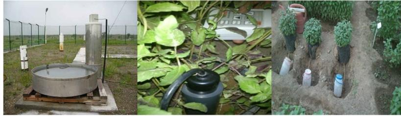
Figure 2. View of the proposed micro-lysimeter, Theta probes, and U.S. class-A pan evaporation methods used in experimental farm
