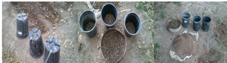
Figure 1. Construction, soil preparation and filling stages in the proposed micro-lysimeter
