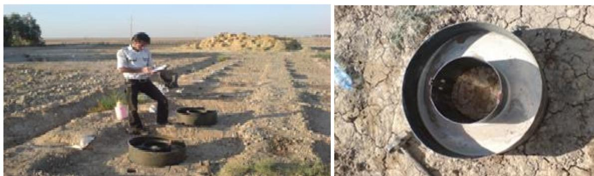
Figure 2. Measuring infiltration by double ring method.
